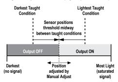
Reverse the CH2 Output ON and OFF conditions by using the LO/DO (Light Operate/ Dark Operate) selection through the program interface.
