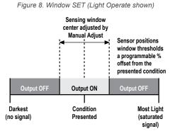
Reverse the Output ON and OFF conditions by using the LO/DO (Light Operate/ Dark Operate) selection through the program interface for the dual output model.
