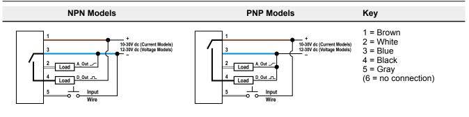
Note: Open lead wires must be connected to a terminal block.
