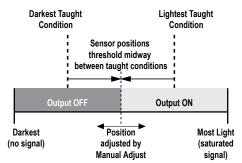
The Output ON and OFF conditions can be reversed by using the LO/DO (Light Operate/ Dark Operate) switch or through the program interface for the dual output model.
